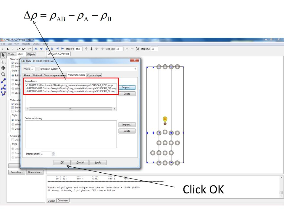
The isosurface of charge density difference is obtained.
